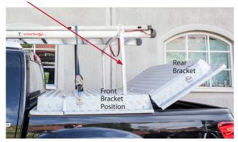
Rack in front position. Medium top load length. The cover can be opened and bed reached.
