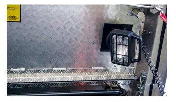
Magnetic foot spootlight with coiled cable. Strong spotlight with protective grille. Excellent for dark environments or night work. Electric wiring is extra if a 12 V socket isn't standard on the pickup.
